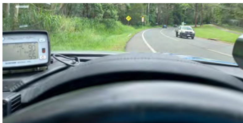
Mobile radar showing the detected speed of a motorbike of 90 km/h in a signed 60 km/h zone.
