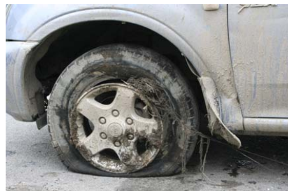
Figure 5: Blown out Left-Front Tire without Rapture
